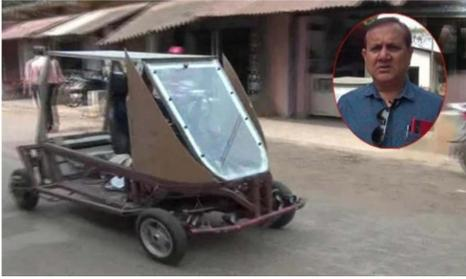
Sushil Aggarwal from Odisha's Mayurbhanj district had built a four-wheeler powered by an 850 Watts motor and 100 Ah/54 Volts of battery. After fully charged the vehicle can travel up to 300 km. They are powered by electricity through the use of solar energy. Sun's energy is directly converted into electrical energy by the Photovoltaic (PV) cells.
